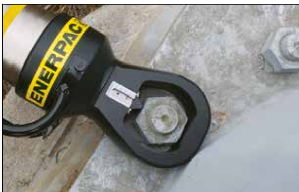
◀ Heavily corroded and weathered nuts are quickly split and removed using a NS-Series Nut Splitter.
