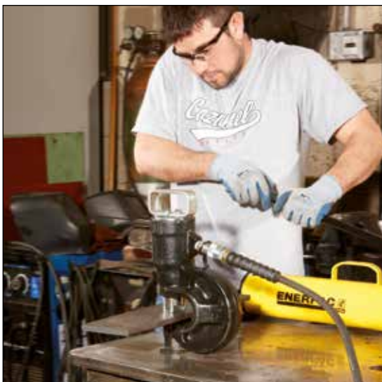
◀ SP-Series, Lightweight Hydraulic Punch – Much Faster than Drilling.
